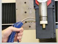
Use compressed air to blow off the coupler threads.
