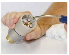
Use compressed air to blow off all internal surfaces.
