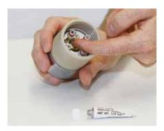
Inspect each of the 5 o-rings at the rear of the torch for nicks and cuts. Replace any damaged o-rings. If they are not damaged, apply a thin film of silicone lubricant on each o-ring. The o-rings should look shiny, but there should not be any excess or built-up grease.
