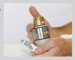
Apply a thin film of silicone lubricant on each external o-ring.
